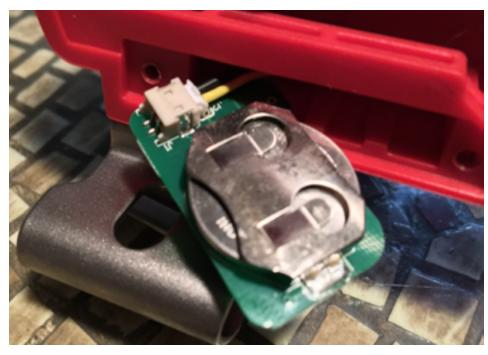
Coin cell is behind a small panel that is underneath where the RedLithium battery attaches
